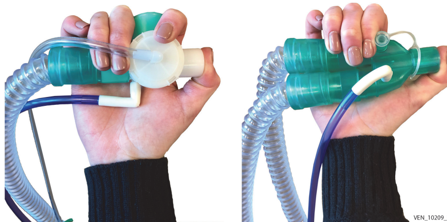
Figure 10-1. Blocking the Patient Circuit (single-limb circuit at left; double-limb circuit at right)
