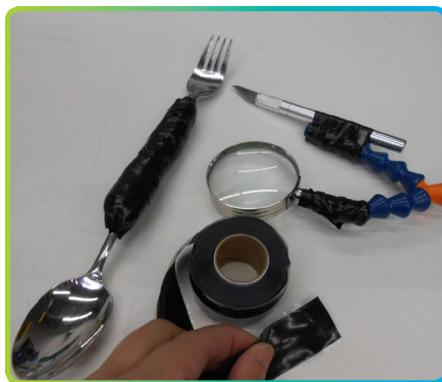
**Silicon Self Adhering Tape** This tape is made, of course, with silicon. To use it, you stretch the tape and wrap it around an object. It then fuses to itself and bonds objects. This tape can be used for many, many purposes: to stop liquid/gas leakage, to hold objects together, to add grips to tools, to insulate electrical wires,
